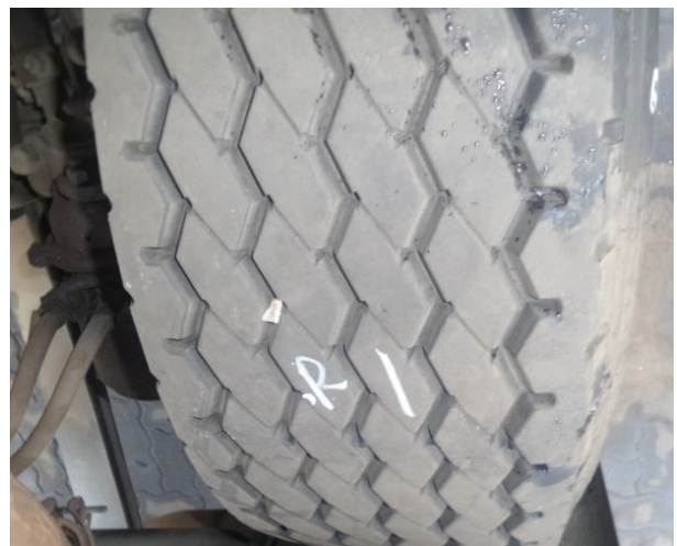
Axle 1 right – roadworthy condition
