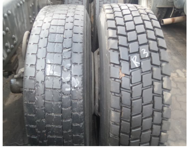
Axle 3 right – roadworthy condition
