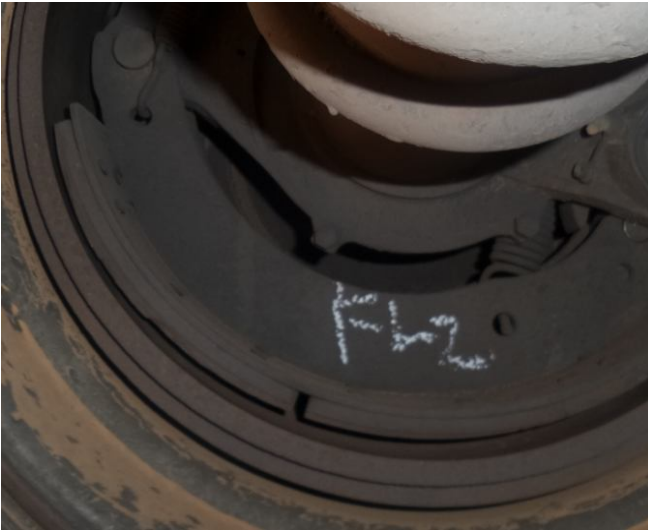
Axle 2 left – adequate linings
