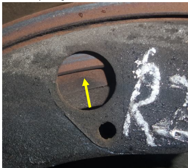
Axle 2 right – adequate linings though overheated
