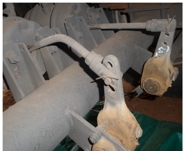
Axle 1 right – pushrod bent
