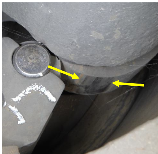
Axle 1 left – excessive roller marks on “S” cam faces
