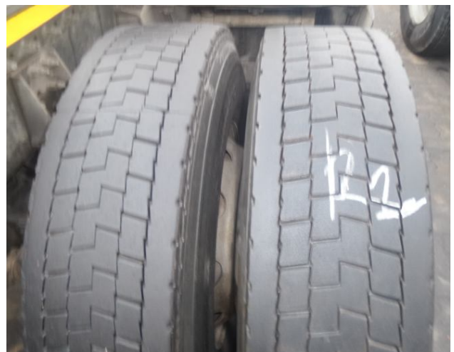
Axle 2 right – roadworthy condition
