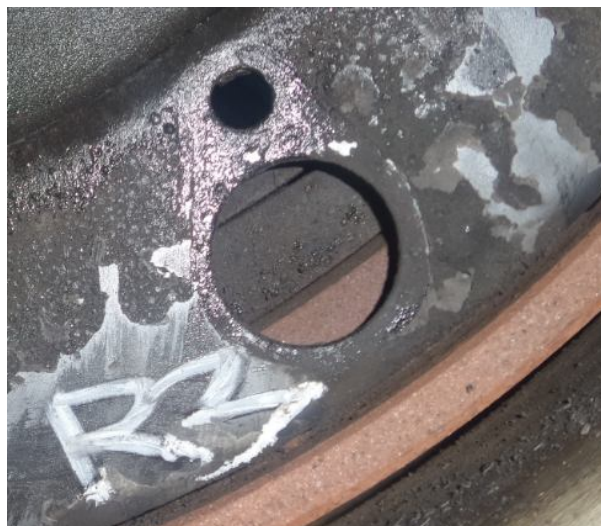
Axle 3 right – overheated brake – paint caught alight
