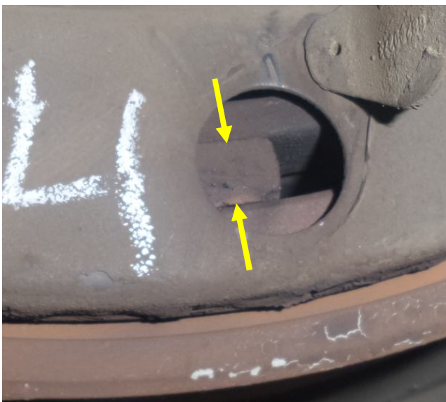
Axle 1 left – adequate linings
