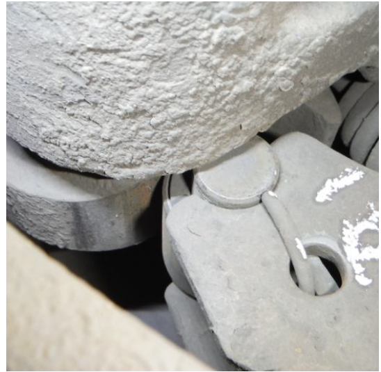
Axle 1 right – excessive roller marks
