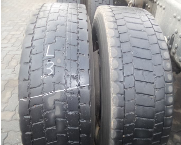
Axle 3 left – outer tyre worn / imminent replacement needed
