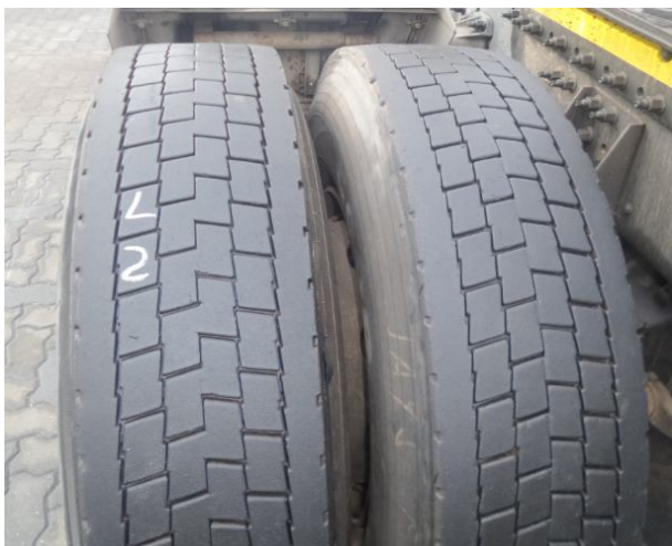
Axle 2 left – roadworthy condition
