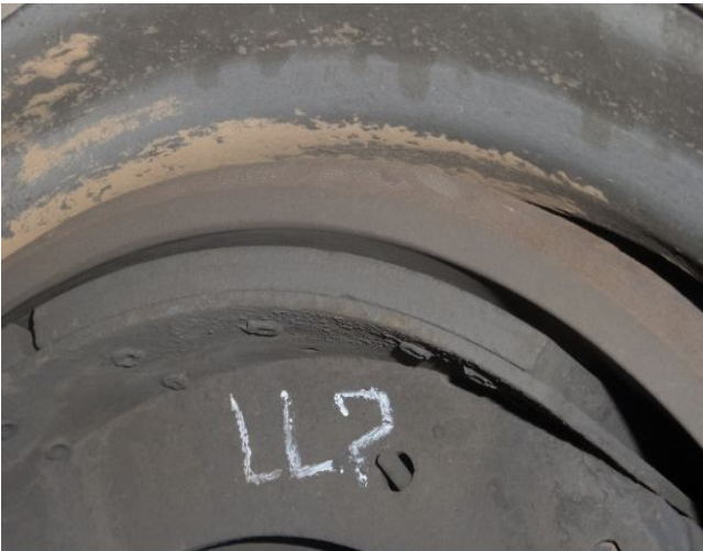
Axle 2 left – adequate linings
