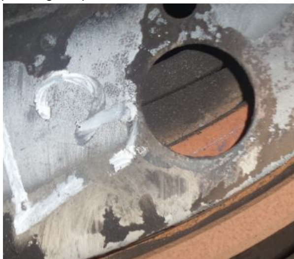
Axle 3 left – overheated brake – paint caught alight
