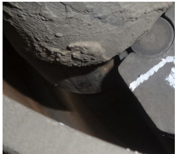
Axle 1 left – excessive roller marks on “S” cam faces
