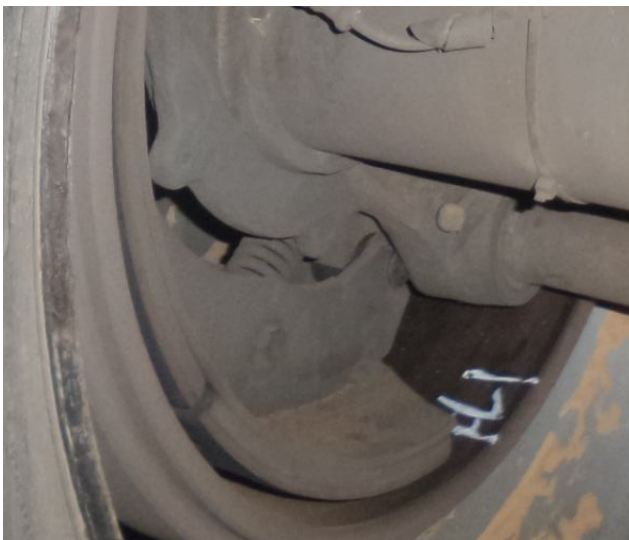
Axle 1 left – adequate linings
