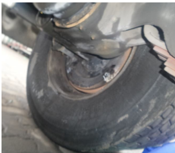
Axle 3 left – overheated brake – paint caught alight
